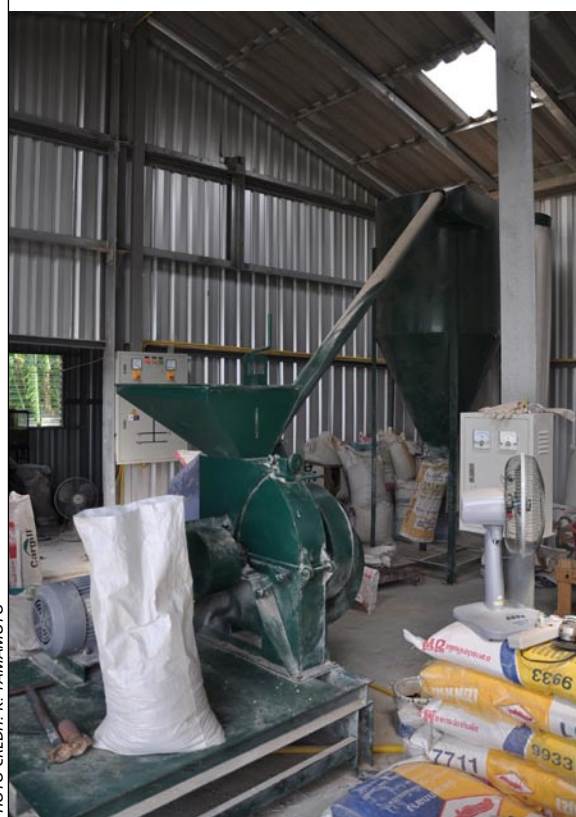
FIGURE 5 Feed mill and semi-floating pellet feed extruder owned and operated by a group of tilapia farmers in Chonburi Province
